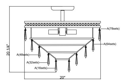
Crystal Sets A. 238 Sets. (1)14mm + (1)60mm plug WARNING: Electrical Danger Turn Power Off
